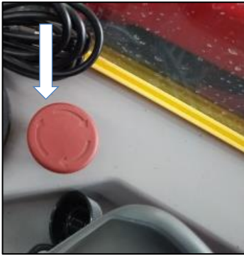
Figure 3.2.4 Emergency stop button
